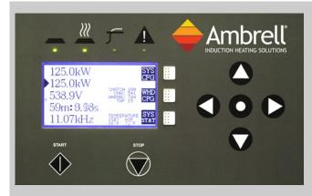
**EKOHEAT** features a front panel programmable controller for monitoring, timer and power-level control, diagnostics and system configuration. Up to 10 ten-step heating profiles can be configured to control power levels over your specified timing requirements.
