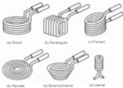
Multiturn coils designed for heating parts of various shapes: (a) round; (b) rectangular; (c) formed; (d) pancake; (e) spiral-helical; (f) internal (from F. W. Curtis, High Frequency Induction Heating , McGraw-Hill, New York, 1950)
